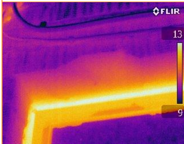
5.26: Thermographic image showing warmer temperature where brickwork is damaged, and leakage around window frame
