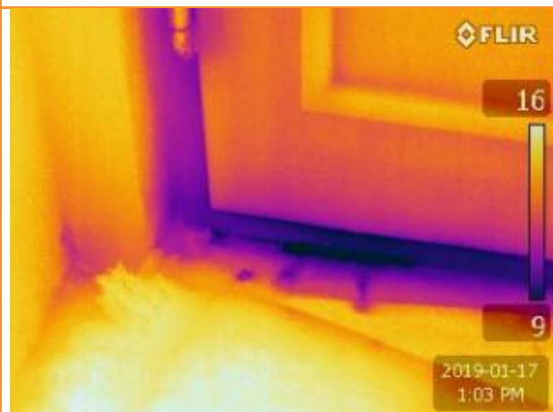
5.01: Internal thermographic image whilst existing house depressurised. Leakage across bottom of glazed door in lounge.
