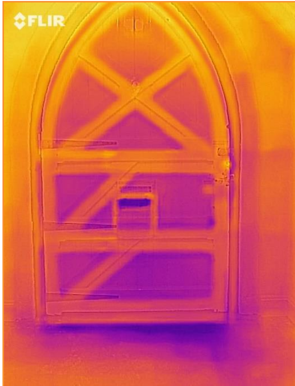
5.14: Internal thermographic image whilst building depressurised, showing substantial cold air (blue) entering the building across the base of the main entrance door, also through the letterbox
