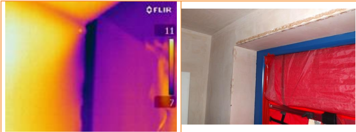
5.18: Thermographic image of cold section formed by leakage along vertical edge of door frame
