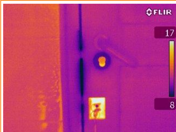
4.22: Thermographic image showing leakage beside kitchen door lock during depressurisation
