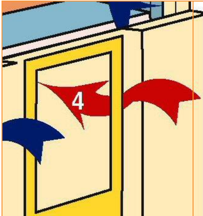
Building Fabric Leakage 4: Through doors – particularly double doors
