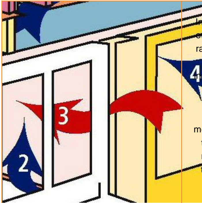
Building Fabric Leakage 3: Through windows joints and/or hollow window frames
