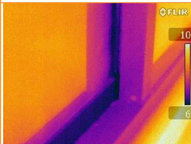
3.20: Thermographic image showing substantial leakage on top floor rear window
