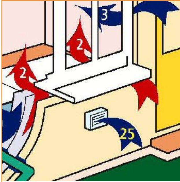
Building Fabric Leakage 2: Beneath window cills and around window frames
