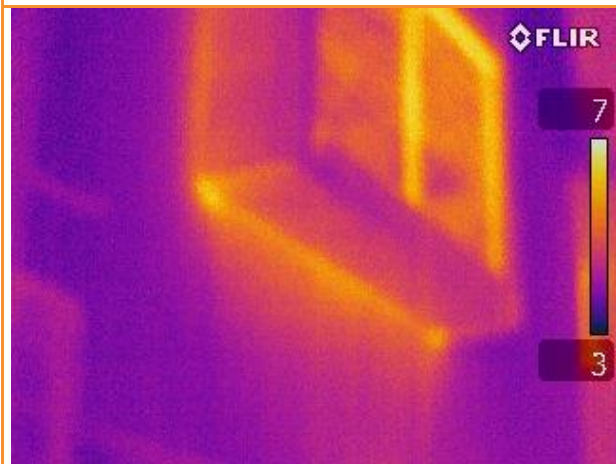
2.53: Thermographic image showing cold bridging and some leakage around projecting window at end of lounge
