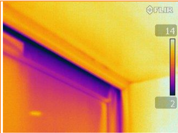
2.42: Internal view of window whilst depressurised, external cold air clearly leaking significantly. Temporary sealing applied to quantify leakage from this source.
