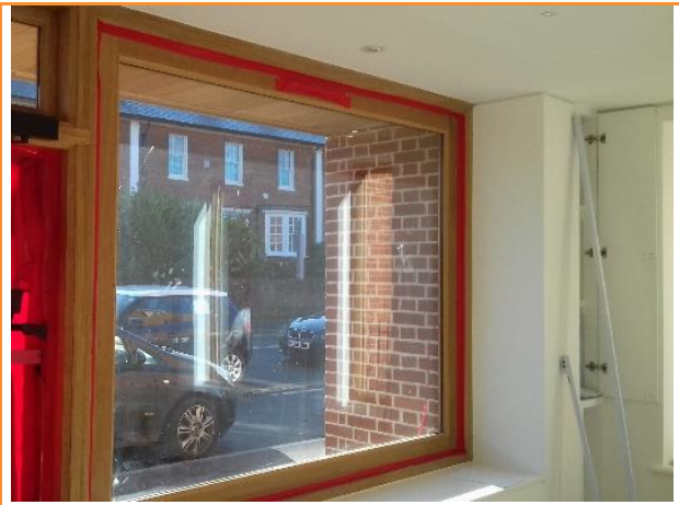
2.42: Internal view of window whilst depressurised, external cold air clearly leaking significantly. Temporary sealing applied to quantify leakage from this source.
