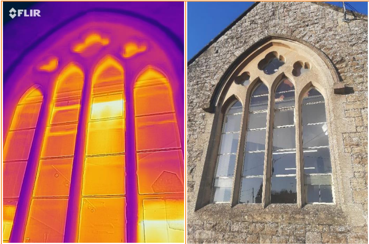
2.26: External thermographic image whilst building pressurised, showing substantial warm air (white/yellow) escaping the building through two windows that don't close properly. Yellow line around the outside of the windows also suggests leakage between the windows and the adjoining stonework, particularly at the top
