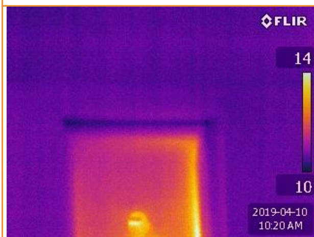
2.37: Thermographic image showing leakage across top of stairwell window
