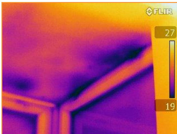
11.02: Thermographic image showing leakage at side of bay window
