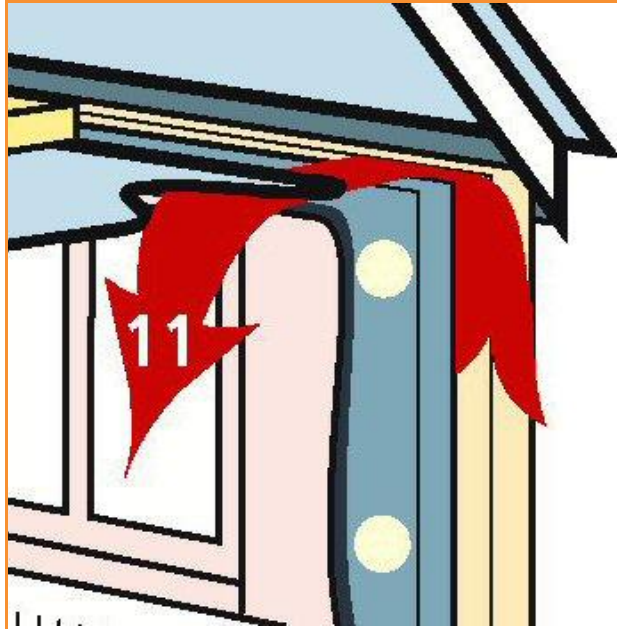
Building Fabric Leakage 11: Through gaps behind plasterboard on dabs or through hollow studwork walls
