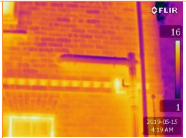
1.02: External thermographic image whilst house is pressurised showing leakage along brick detail at intermediate floor level.
