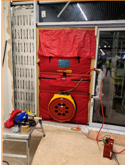
A1.1) Internal view of test equipment mounted in bag door system in L1 Main Entrance
