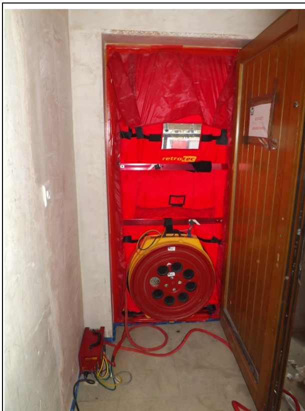
P3) Test equipment mounted in front doorway
